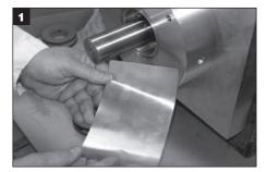
Cut 0.005" thick brass shim stock approx. 1/4" larger than circumference of the shaft.
