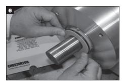
Remove the shim and uniformly press the seal into the bore.
