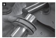
Roll the shim stock and carefully pass through the seal.
