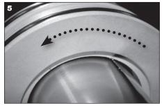
Rotate the seal in the direction of the shim overlap and slide over the shaft.
