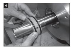
Position the shim and the seal over the shaft.
